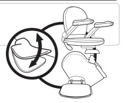
To turn the seat, depress and hold down the seat swivel lever at the side of the seat pad. This will then allow the seat to be rotated to face the staircase landing. The seat will lock in position at 45° and 90°.
