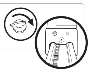
The display panel, positioned near the key switch, will indicate 'A1', or 'C1, C2, C3, C4, C5 or C6' if the stairlift is on a charge point.
