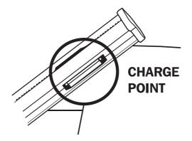
Note: If there is a mains electrical supply failure, or if the supply to your stairlift is switched off, it will continue to work for several journeys. However, the batteries will eventually lose their charge and the stairlift will not operate.
